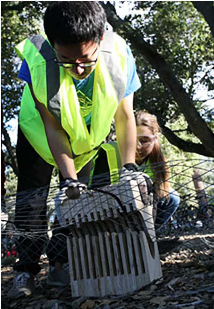
Figure 4a: COCOON: Stamping the truss patterns with plywood molds
